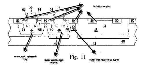
each outer well region has an upper surface which includes a source/drain region 60/62 (col. 4, lines 57-67); a field effect transistor having at least a gate conductor 58 of the first conductivity type located above the inner well region 46; and wherein the outer well regions 44/52 and the inner well region 46 are in contact with the subcollector 42 (col. 4, line 67 to col. 5, line 6 and FIG. 11).
